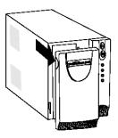
2. Slide up and remove the metal battery cover.
